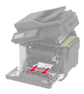
**3** Open the fuser access door, and then remove the jammed
